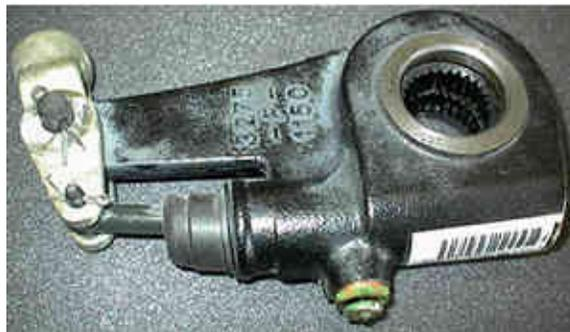
Figure 5: Automatic slack adjuster example
