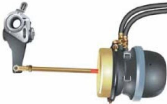
Figure 3: Brake chamber pushrod indicator
