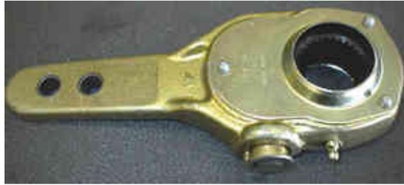
Figure 4: Manual slack adjuster example
