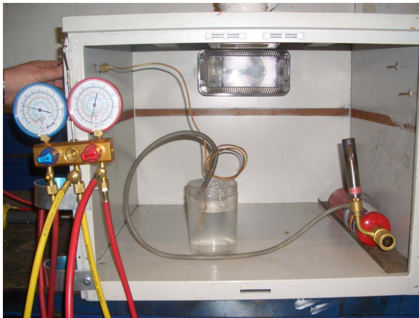
Photo F - Example of test set-up using manifold gauge set
