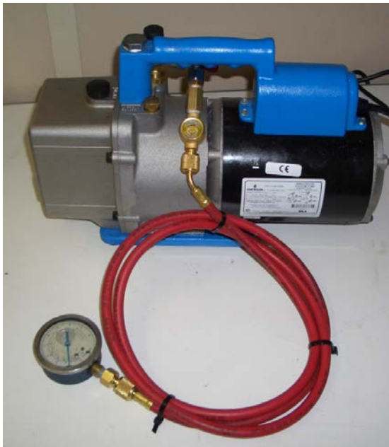
Rig connected to vacuum pump
