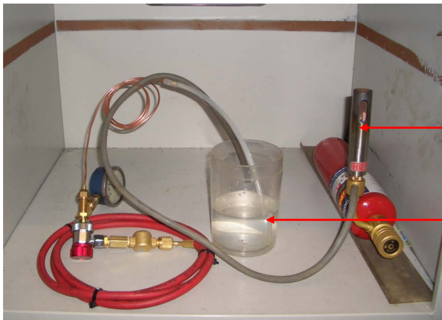
Photo E - Example of test set-up using fume cupboard with extractor fan
