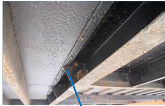
Tunnel bolster Gusset RLG
