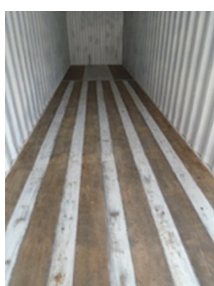
Steel-wood combination Omega floor design (Photo: Institute of International Container Lessors)
