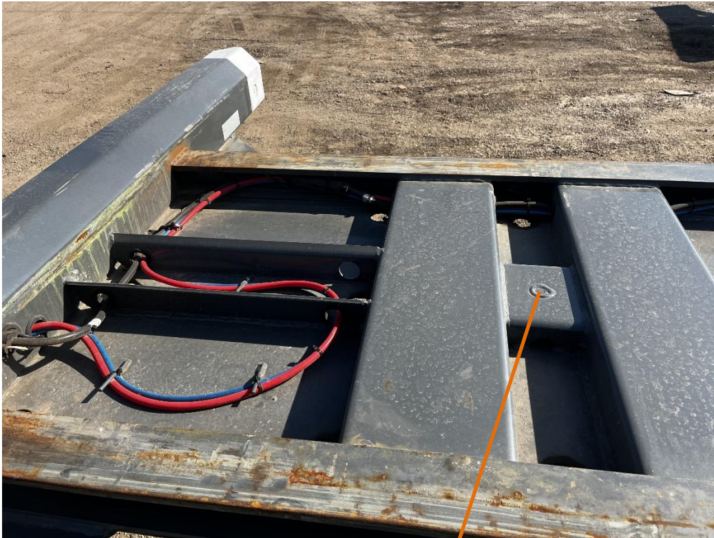
Kingpin Reinforcement Framing KKT
