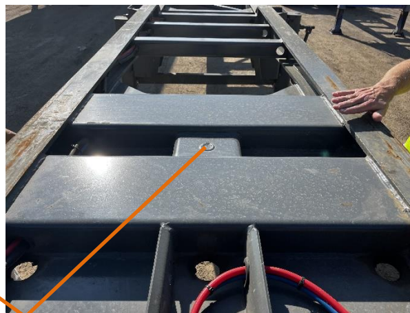
Kingpin Reinforcement Framing KKT
